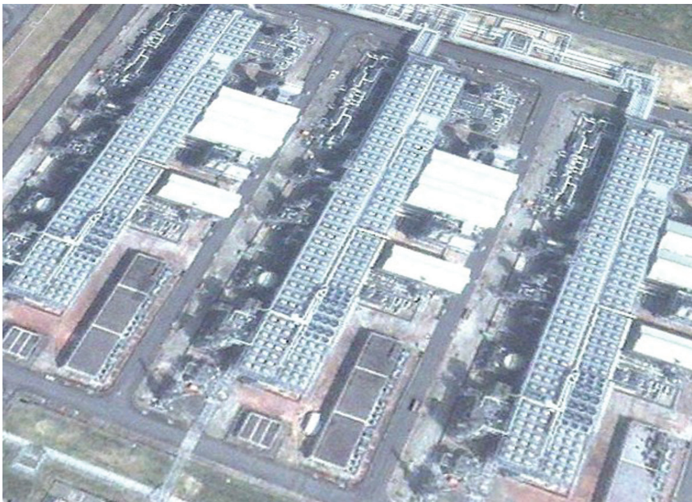
Figure 1: Large air cooled heat exchanger trains in Nigeria LNG Plant, from Google Earth
