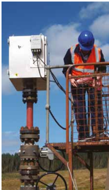
Figure 1. Prototype LineGate on test at DNV GL facility at Spadeadam. Note: The long vertical section simulates the distance to a buried pipeline
