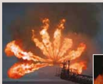
Offshore liquid burners • Multipoint -burners pointing in different directions
